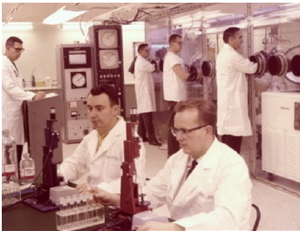
Figure 65. Containment System in Bldg. K-703 at Oak Ridge (Circa 1963)
