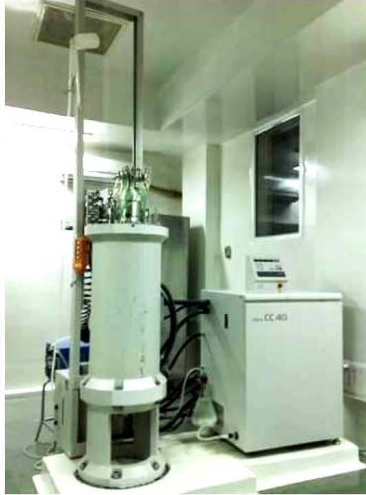
Figure 9. Commercial Installation of the CC-40 Centrifuge
